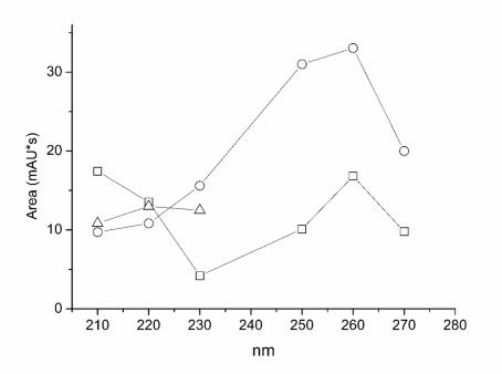
Figure 2. The effect of the wavelength on the peak areas of benzoic acid ( $\triangle$ ), sorbic acid ( $\bigcirc$ ) and cinnamic acid ( $\square$ ). Running buffer, 20 mM Borate, pH 9.3; injection, 4 s at 50 mbar; run voltage, 28 kV
