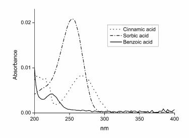
Figure 1. Spectra of benzoic, sorbic and cinnamic acid
